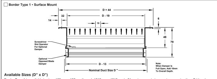
Border Type 1 is available in sizes 152mm x 102mm through 1219mm x 1219mm in 51mm increments in one piece construction. Odd and fractional sizes are available at additional cost. Sizes larger than 1219mm x 1219mm are shipped in multiple sections with joining strips for field
