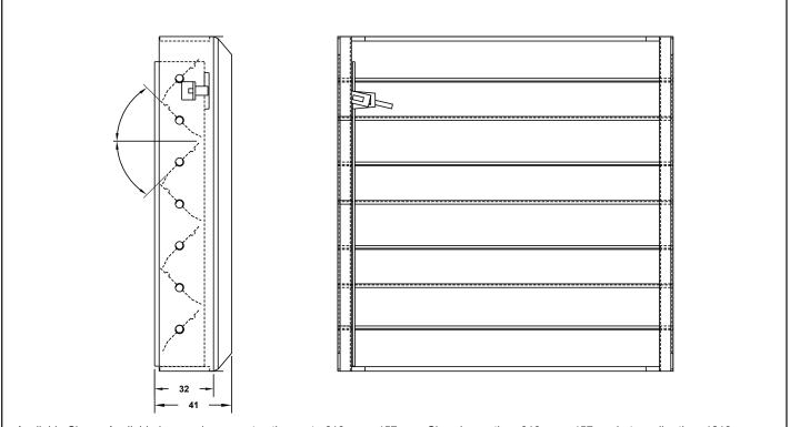
Available Sizes: Available in one piece construction up to 610mm x 457mm. Sizes larger than 610mm x 457mm but smaller than 1219mm x 1219mm are made in multiple sections and shipped as one piece. Dimensions are in millimeters.
