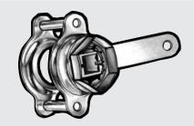
The Young 443 3/8" lever-type Valcalox regulator is similar to our 403 regulator except that it has a base 1" in depth designed for mounting on externally insulated duct. All 443 series regulators are operated by our 04 wrench, available separately.
