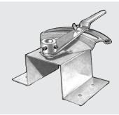
The 404 lever type quadrant will control dampers with a  $\frac{1}{2}$ " round shaft. Constructed of plated steel with set screws and lock washer with a die cast handle. Pictured is the 404B, a 404 on a 2" base for insulated duct.
