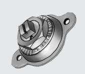
The Young 401 Valcalox self-locking regulator for 3/8" square damper shaft is designed to be mounted directly on the surface of a round or rectangular duct where the damper is located. It may be used with Young 820A-L rectangular or 5020 round dampers, as well as with other manufacturers' dampers that have 3/8" square shafts.
