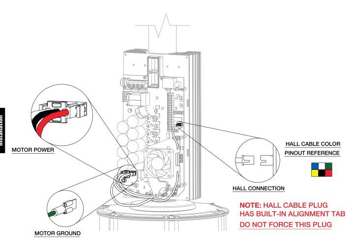
**Motor Power and Ground Cable Connection**
