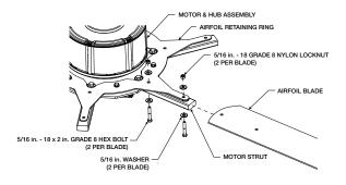
Repeat steps 1 through 3 on remaining airfoil blades. Torque the installed bolts to 25 ft·lbf (34 N·m).
