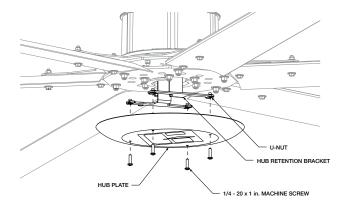
**IMPORTANT:** Rotate fan impeller by hand to ensure that it rotates freely and does not rub on hub plate or come into contact with any obstructions.
