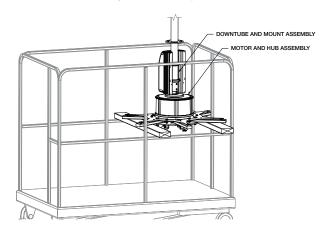
Install the supplied (2) 3/8 in. – 16 x 2-3/4 in. grade 8 hex bolts into the locknuts attached to the downtube. Torque the bolts to a value of 33 ft·lbf (44.75 N·m).
