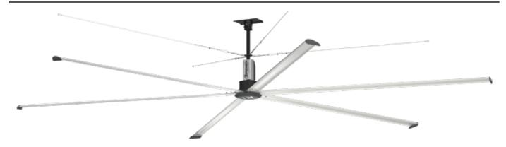
AMPLIFY™ Models DS-3 and DS-6 are the ideal choice for providing year-round comfort in air circulation and destratification applications. Featuring an aerodynamic, extruded aluminum airfoil design and a high efficiency direct drive motor, model DS delivers maximum airflow at a fraction of the operating cost of other HVLS fans. And, with its universal ceiling mount, the DS fan is the easiest HVLS fan to install in the market!
