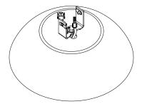
NOTE: The LED light assembly can be pivoted out of the way to simplify connection of the light power and light communication plugs.
