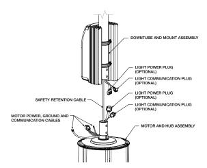
4. Carefully align the motor axle with the downtube opening, making sure that the electrical cables protruding from the motor axle are on the same side as the black plastic VFD cover.
