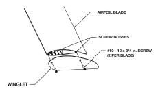
**NOTE:** Improperly fastened winglets may result in unwanted noise.
