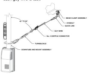
4. Place a level against the downtube and tighten all (4) turnbuckles by hand in a crisscross pattern until the guy wires are tight and the fan is level.
