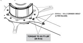
**IMPORTANT:** If airfoils must be removed and reinstalled for any reason, do not re-use the supplied nylon locknuts. Re-use increases the risk of locknuts loosening during operation, which may result in unwanted noise and/or unsafe operation of the fan. Contact your local representative or the factory if replacement parts are needed.
