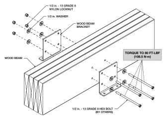
3. With wood beam brackets installed, line up universal mounting plate and bolt into wood beam brackets using supplied (4) 1/2 in. – 13 x 1-1/2 in. hex bolts, (8) 1/2 in. washers, and (4) 1/2 in. – 13 nylon locknuts.
