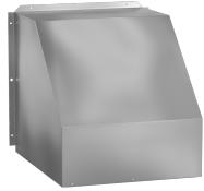
Weatherhoods shield wall openings and dampers from rain and snow. Weatherhoods are shipped unassembled in kit form for field assembly. Construction is of galvanized steel with wire mesh birdscreen.
