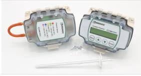
The Constant Pressure Control can be used to monitor static pressure in a system, automatically adjusting the fan speed to maintain a desired static pressure. This control reduces energy consumption not only by reducing the speed and the energy used by the fan, but will also reduce the amount of conditioned air that is exhausted. Recommended for use in multi-family structures, hotels and schools where demand control ventilation applications exist.
