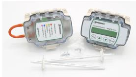
The Constant Airflow Control is used to monitor velocity pressure in a system, automatically adjusting the fan speed to maintain a desired velocity pressure (constant CFM). This control reduces energy consumption not only by reducing the speed and the energy used by the fan, but will also reduce the amount of conditioned air that is exhausted. Recommended for use in multi-family structures, hotels and schools where demand control ventilation applications exist.
