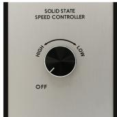
Speed controls are used for manual adjustment of the fan's performance (for final system balancing) or to control the fan's output in confined spaces, such as conference or meeting rooms. The fan can be adjusted to 60% of design airflow with a speed control. This reduction in airflow and fan speed is also accompanied by a reduction in noise level. Note: For use on direct drive fans with single phase, PSC or shaded pole motors.
