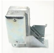
Model MP-310 is a damper actuator pack used to convert the WD-300 series backdraft damper to motorized operation. These versatile motor packs feature power opening with spring return. The springs also provide damper closure in the event of electrical failure. MP-310 is supplied with mounting hardware, assembly instructions and actuator arms for either single, double, or triple panel installation. Rated for 460V. UL listed.
