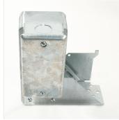
Model MP-310 is a damper actuator pack used to convert the WD-300 series backdraft damper to motorized operation. These versatile motor packs feature power opening with spring return. The springs also provide damper closure in the event of electrical failure. MP-310 is supplied with mounting hardware, assembly instructions and actuator arms for either single, double, or triple panel installation. Rated for 115-230V. UL listed.
