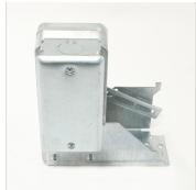
Model MP-200 is a damper actuator pack used to convert the WD-200 series backdraft damper to motorized operation. These UL listed motor packs use single phase 60hz shaded pole stall type impedance protected electric actuators. MP-200 is supplied with mounting hardware, assembly instructions and actuator arms for either single, double, or triple panel installation. Rated for 460V.
