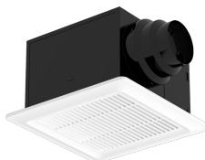
Model SP-AP features a virtually silent electronically commutated (EC) motor with three built-in, high-speed airflow settings (50, 80 or 110 cfm) and a handful of plug and play sensors available as add-ons.
