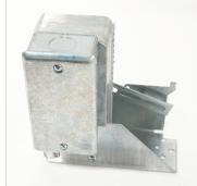
Model MP-200A/MP-220A is a damper actuator pack used to convert the WD-200 series backdraft damper to motorized operation. These UL listed motor packs use single phase 60hz shaded pole stall type impedance protected electric actuators. MP-200A/MP-220A is supplied with mounting hardware, assembly instructions and actuator arms for either single, double, or triple panel installation. Rated for 115-230V.
