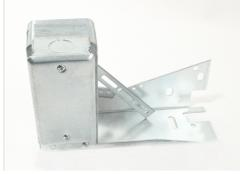
Model MP-100A is a damper actuator pack used to convert the WD-100 horizontal mount backdraft damper to motorized operation. These versatile motor packs feature power opening with spring return. The springs also provide damper closure in the event of electrical failure. MP-100A motor packs are supplied with mounting hardware, assembly instructions and actuator arms for either single or double panel installation. Rated for 24V. UL listed.
