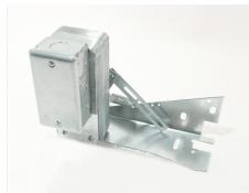
Model MP-100A is a damper actuator pack used to convert the WD-100 horizontal mount backdraft damper to motorized operation. These versatile motor packs feature power opening with spring return. The springs also provide damper closure in the event of electrical failure. MP-100A motor packs are supplied with mounting hardware, assembly instructions and actuator arms for either single or double panel installation. Rated for 115-230V. UL Listed.
