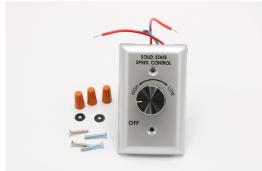
Speed controls are used for manual adjustment of the fan's performance (for final system balancing) or to control the fan's output in confined spaces, such as conference or meeting rooms. The fan can be adjusted to 60% of design airflow with a speed control. This reduction in airflow and fan speed is also accompanied by a reduction in noise level. Note: For use on direct drive fans with single phase, PSC or shaded pole motors.
