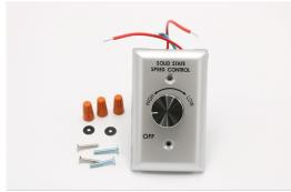
Speed controls are used for manual adjustment of the fan's performance (for final system balancing) or to control the fan's output in confined spaces, such as conference or meeting rooms. The fan can be adjusted to 60% of design airflow with a speed control. This reduction in airflow and fan speed is also accompanied by a reduction in noise level. Note: For use on direct drive fans with single phase, PSC or shaded pole motors.
