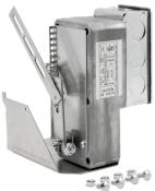
Model MP-210 is a damper actuator pack used to convert the WD-200 series backdraft damper to motorized operation. These UL listed motor packs use single phase 60hz shaded pole stall type impedance protected electric actuators. MP-210 is supplied with mounting hardware, assembly instructions and actuator arms for either single, double, or triple panel installation. Rated for 24V.
