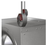
Complete hanging isolation kit with spring isolators to reduce vibration and sound levels. Support brackets included are designed to permit mounting of the fan with the motor located on top, bottom or side.
