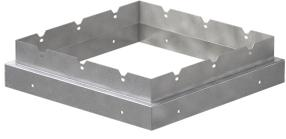
Curb adapters are designed to adapt standard curb cap dimensions to existing curb when replacing a fan or ventilator. Constructed of galvanized steel. For use with model AE, sizes 12 through 14, model AS, sizes 12 through 14, model CUBE, sizes 141 through 161, model CUE, sizes 141 through 161, model G, sizes 143 through 163, and model GB, sizes 141 through 161.
