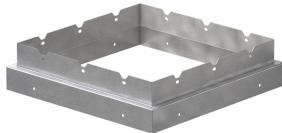
Curb adapters are designed to adapt standard curb cap dimensions to existing curb when replacing a fan or ventilator. Constructed of galvanized steel. For use with AE-10, AS-10, CUBE models, sizes 099 through 131, CUE models, sizes 080-099 and GB models, sizes 071 through 131.
