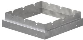
Curb adapters are designed to adapt standard curb cap dimensions to existing curb when replacing a fan or ventilator. Constructed of galvanized steel. For use with CUE models, sizes 060 through 070, and G models, sizes 060 through 095.
