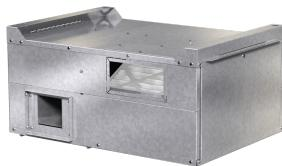
The MiniVent is an energy recovery ventilator designed for indoor installations in commercial and institutional applications. The compact design provides an economical solution for individual spaces, such as school classrooms and small offices and may be floor mounted or ceiling hung. A removable panel enables easy access to filters and enthalpy wheel.
