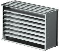
Brick vents provide a permanent means of ventilation for crawl spaces, hung ceilings, incinerator rooms, chimney flues, foundations, pipe spaces and corridors. Extruded construction provides a quality finished appearance. A high water stop at the rear and deep overlapping blades with storm stops provide maximum resistance to rain and weather.
