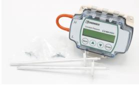
The Constant Airflow Control is used to monitor velocity pressure in a system, automatically adjusting the fan speed to maintain a desired velocity pressure (constant CFM). This control reduces energy consumption not only by reducing the speed and the energy used by the fan, but will also reduce the amount of conditioned air that is exhausted. Recommended for use in multi-family structures, hotels and schools where demand control ventilation applications exist.
