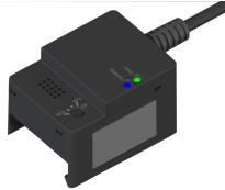
The plug-in integrated dehumidistat automatically detects excess humidity in a space and activates the fan for control of excess moisture. The sensitivity is adjustable from 50% RH to 80% RH and also includes a built in 15 minute time delay.
