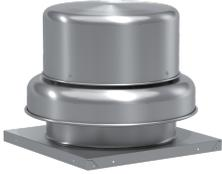
Model GB, belt drive centrifugal roof exhaust fans are designed to meet the general clean air exhaust requirements for industrial and commercial buildings. Units feature a fully rolled windband bead for increased stability and easy transport. Fresh outside air is drawn in under the motor cover to maximize motor life.
