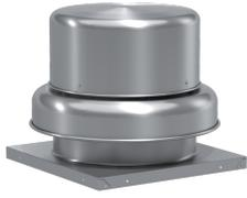
Model GB, belt drive centrifugal roof exhaust fans are designed to meet the general clean air exhaust requirements for industrial and commercial buildings. Units feature a fully rolled windband bead for increased stability and easy transport. Fresh outside air is drawn in under the motor cover to maximize motor life.
