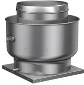
The CUBE is an aluminum exhaust fan specifically designed for roof or sidewall mounted applications where contaminated or grease laden exhaust air can be discharged directly upward, away from the roof or wall surface. The fans feature a one piece windband continuously welded to curb cap and double studed isolators for true vibration isolation.
