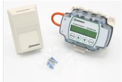
The Constant Pressure Control can be used to monitor static pressure in a system, automatically adjusting the fan speed to maintain a desired static pressure. This control reduces energy consumption not only by reducing the speed and the energy used by the fan, but will also reduce the amount of conditioned air that is exhausted. Recommended for use in multi-family structures, hotels and schools where demand control ventilation applications exist.
