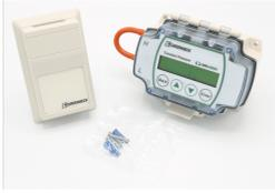
The Constant Pressure Control can be used to monitor static pressure in a system, automatically adjusting the fan speed to maintain a desired static pressure. This control reduces energy consumption not only by reducing the speed and the energy used by the fan, but will also reduce the amount of conditioned air that is exhausted. Recommended for use in multi-family structures, hotels and schools where demand control ventilation applications exist.
