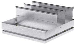
The BD-100 is a horizontal mount backdraft damper designed to allow vertical airflow up and prevent reverse airflow. The dampers are opened by air pressure differential (assisted by springs) and closed by gravity. The damper features a flangeless, galvanized steel frame with aluminum blades.
