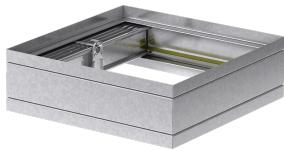
The SP Ceiling Radiation damper protects fire rated ceilings and effectively blocks the spread of heat and flames through the building's ventilation system. This damper is UL Classified; rated at three to four hours fire resistance. For use with Lighted SP Fans.
