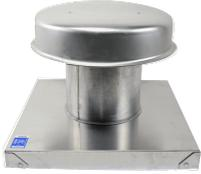
Model RCC-7 roof cap accessory includes weathertight aluminum construction with an integral birdscreen and built-in curb cap. Requires roof curb (sold separately).
