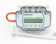
The Constant Pressure Control can be used to monitor static pressure in a system, automatically adjusting the fan speed to maintain a desired static pressure. This control reduces energy consumption not only by reducing the speed and the energy used by the fan, but will also reduce the amount of conditioned air that is exhausted. Recommended for use in multi-family structures, hotels and schools where demand control ventilation applications exist.
