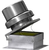
Hinge kit allows the fan to hinge at the base of the curb cap for access to the wheel and ductwork for inspection and cleaning.
