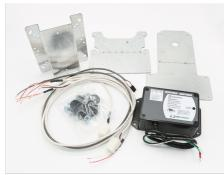
The Vari-Green transformer provides a 24-volt power source from the existing line voltage at the fan to the motor and controls. It has two dry auxiliary contacts (one normally open and one normally closed) available to signal a motorized damper or interlock with other devices.
