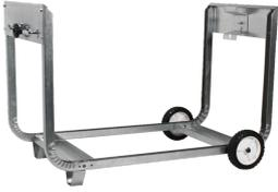
The tilttable carriage provides a stable, portable carriage that can be easily rolled about in industrial environments. Constructed of steel and includes assembly hardware and carriage with quick-turn knobs for easy tilt adjustment and multi-directional airflow.
