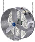
Designed to mount Model MAC to ceiling beams or rafters in industrial environments. Kit includes heavy-duty 3-point attachments allowing easy tilt adjustment and multi-directional airflow.
