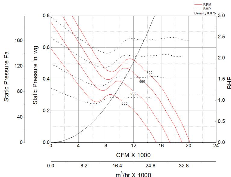
Note: The maximum FRPM for each motor horsepower is shown. For additional performance ranges available for this fan, refer to the performance table.
