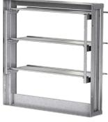
The WD-330 series dampers are designed to prevent reverse airflow in horizontal exhaust applications. The WD-330 features a pressure sensitive blade design that opens and remains open under low velocity conditions. The dampers are opened by air pressure differential and closed by gravity. Galvanized steel, flangeless frame.
