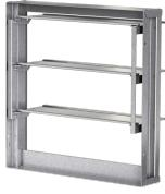
The WD-330 series dampers are designed to prevent reverse airflow in horizontal exhaust applications. The WD-330 features a pressure sensitive blade design that opens and remains open under low velocity conditions. The dampers are opened by air pressure differential and closed by gravity. Galvanized steel, flangeless frame.
