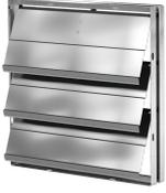
The BD-330 is a vertical mount backdraft damper designed to allow horizontal airflow and prevent reverse airflow. The dampers are opened by air pressure differential and closed by gravity. The damper features a flangeless, galvanized steel frame with aluminum blades.
