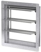
The WD-320 series dampers are designed to prevent reverse airflow in horizontal exhaust applications. The WD-320 features a pressure sensitive blade design that opens and remains open under low velocity conditions. The dampers are opened by air pressure differential and closed by gravity. Galvanized steel frame with flange on the discharge side.
