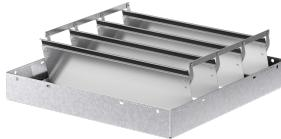
The WD-100 series are horizontally mounted backdraft dampers designed to allow vertical airflow up and prevent reverse airflow. The dampers are opened by air pressure differential (assisted by springs) and closed by gravity. The damper features a flangeless, galvanized steel frame and aluminum blades.
