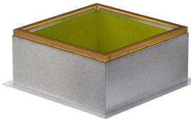
GPI roof curbs are designed for flat, insulated or non-insulated roof decks. Constructed of 18 gauge galvanized steel and fully formed on three sides with a single, fully welded seam.
