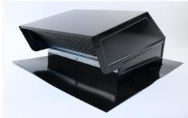
Pitched roof cap discharge accessory constructed of steel with black enamel finish. Includes integral flashing, flash, built-in birdscreen and damper.
