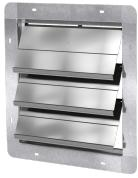
The BD-320 is a vertical mount backdraft damper designed to allow horizontal airflow and prevent reverse airflow. The dampers are opened by air pressure differential and closed by gravity. The damper features a galvanized steel frame with a flange on the discharge side and aluminum blades.
