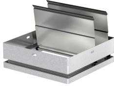
The BD-90 is a horizontal mount backdraft damper designed to allow vertical airflow up and prevent reverse airflow. The dampers are opened by air pressure differential and closed by gravity. The damper features a flangeless, galvanized steel frame and aluminum blades.
