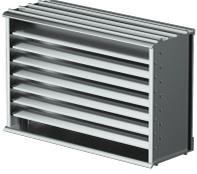
Brick vents provide a permanent means of ventilation for crawl spaces, hung ceilings, incinerator rooms, chimney flues, foundations, pipe spaces and corridors. Extruded construction provides a quality finished appearance. A high water stop at the rear and deep overlapping blades with storm stops provide maximum resistance to rain and weather.
