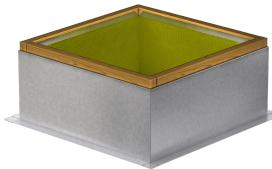
GPI roof curbs are designed for flat, insulated or non-insulated roof decks. Constructed of 18 gauge galvanized steel and fully formed on three sides with a single, fully welded seam.
