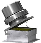
Hinge kit allows the fan to hinge at the base of the curb cap for access to the wheel and ductwork for inspection and cleaning.
